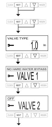
When VALVE TYPE screen appears, press NEXT to go to the VALVE 1 screen.
