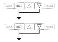
When VALVE TYPE screen appears, press NEXT to go to the VALVE 1 screen.
